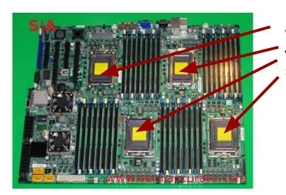
arya.int-evry.fr 4 sockets with 12 cores in each socket => 48 cores in total
