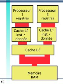
Architecture *Multi-core* (ex. Intel Dual/Quad core, Cell)
